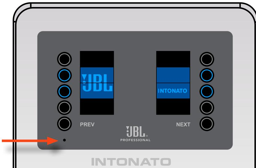
3. Select the desired menu option using the **OPTION** buttons to the left of the display.
