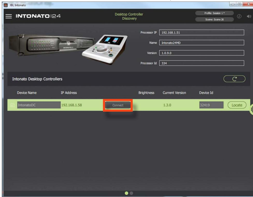
5. Select the desired LCD and button brightness using the **Brightness** dropdown menu (4=brightest, 1=dimmest). In most cases, it is recommended that a high Brightness setting be used (e.g., 4), as this will allow a higher contrast between active and inactive LED states.
