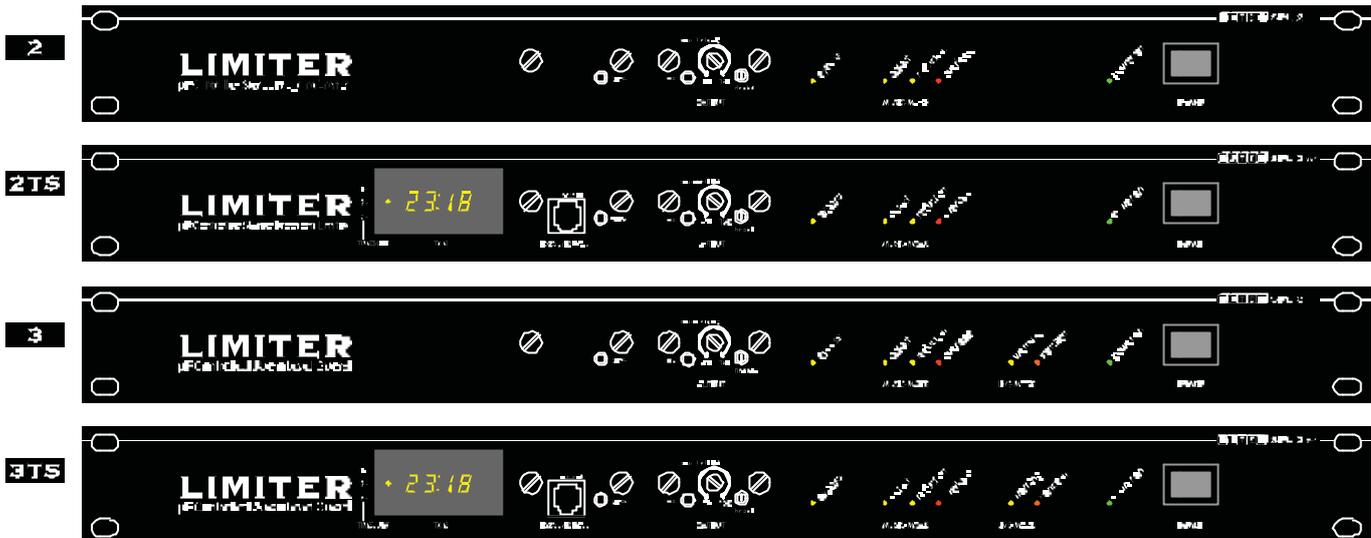
The SPL2, SPL2TS, SPL3 and SPL3TS are sound pressure limiters (SPL), especially designed for use in public houses, discotheques, etc. The SPL-limiters are no peak-limiters, they only limit the average sound pressure. Trimmers for on-site calibration are positioned behind removable cover(plates) which can be put under seal.
