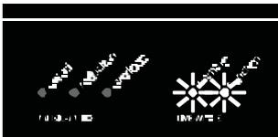
WARNING- & SANCTION-LED (11)(12) blinking: the supplied microphone is not connected correctly. Check the connection.
